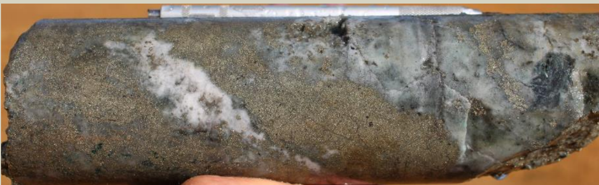
Massive sulphide-quartz veining replacing ultramafic protolith at 168.5m.
