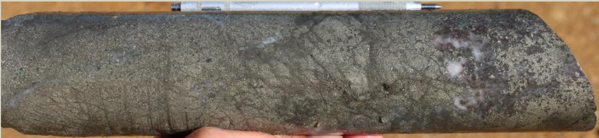
Massive sulphide-quartz veining at 153.8m.
