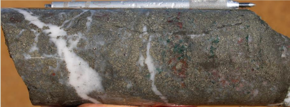
Massive sulphide-quartz veining with trace hematite and fucsite at 144.2m.
