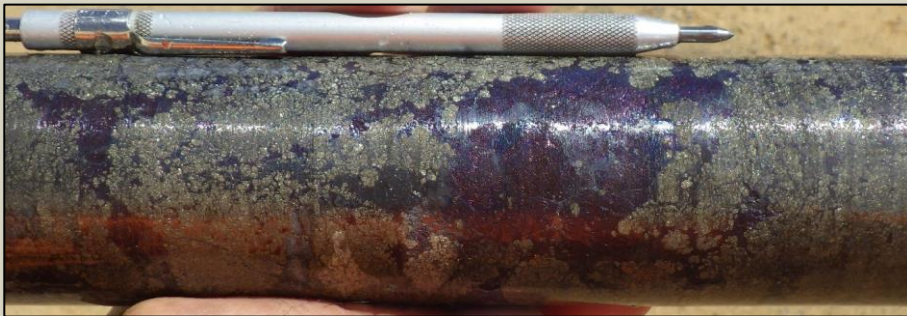
Photo 2. Chalcocite(±digenite)-bornite-covellite veining at 859.0m in SMD044W1 (This photo is of the other side of the core in the previous photo).
